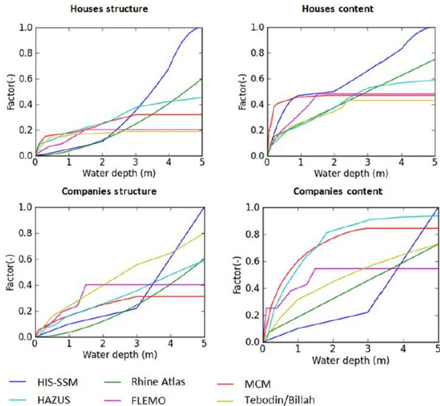
Figure 2-4 Average damage functions for the different flood damage models in the damage function library. Blue: HIS-SSM, green: Rhine Atlas, red: MCM, light blue: FLEMO, pink: HAZUS, yellow: Billah (2007) for houses and Tebodin for companies (Wagenaar et. Al, 2016)
