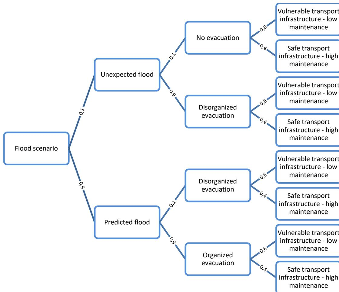
Figure 2-8 Event tree - Four different partial evacuation scenarios and the link to transport infrastructure condition (adjusted from Rijkswaterstaat VNK Project Office, 2014)
